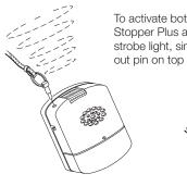
To activate both Mugger Stopper Plus alarm and strobe light, simply pull out pin on top of unit.
