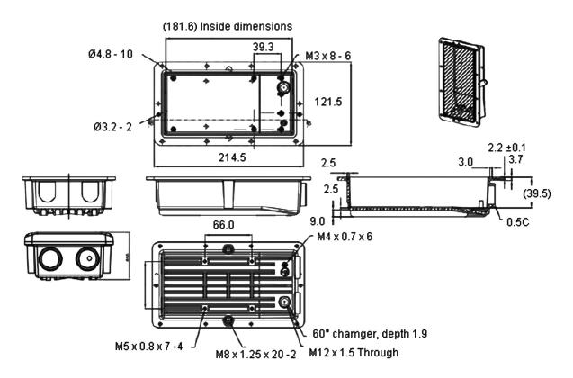
A highly customizable IP67 rated enclosure designed for wireless and industrial control systems in harsh environments. IP67 protection, total protection against dust ingress and the water ingress (water immersion up to 1 meter).
