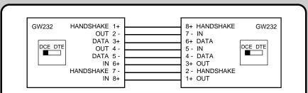
Diagram of two GW232 units connected in 8 wire Data and handshake configuration, extending the RS-232 interface. Full duplex serial channel with hardware handshaking.
