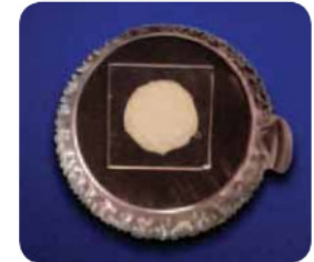
After 300 Cycles: Remains tacky with zero pump out
