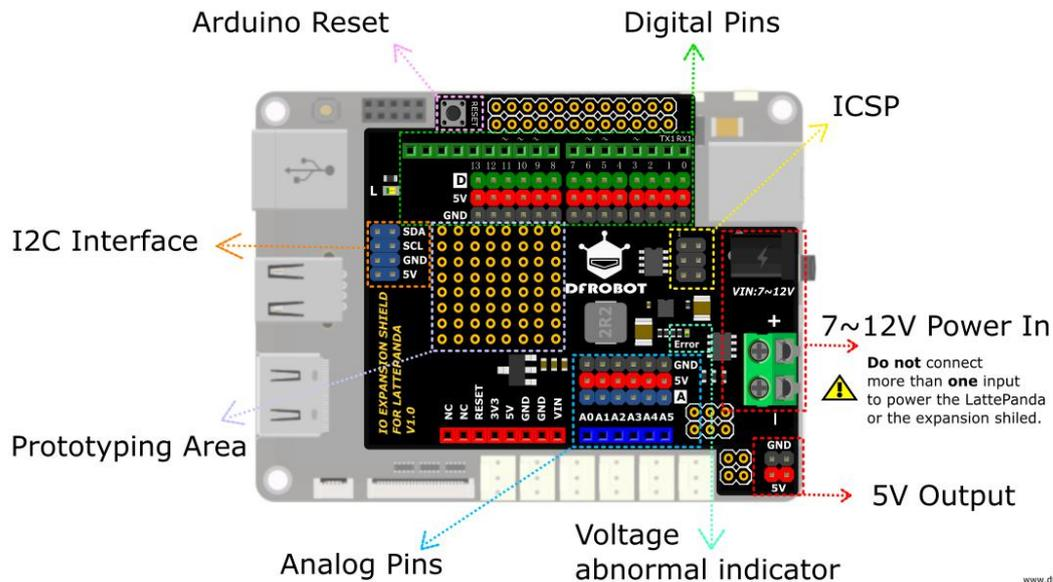
Gravity IO Expansion Shield for LattePanda Pinout
