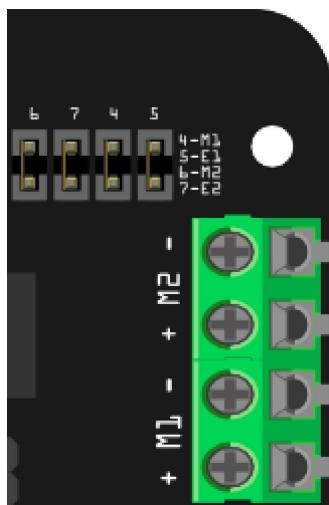
The PWM DC motor control is implemented by manipulating two digital IO pins and two PWM pins. As illustrated in the diagram above (Figure 5), Pin 4,7 (7,8 for old Romeo version) are motor direction control pins, Pin 5,6 (6,9 for old Romeo version) are motor speed control pins.
