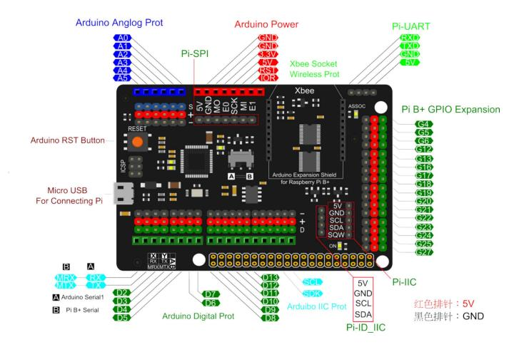
**NOTE**: The ID-I2C is an EEPROM interface, which is dedicated to connect to external EEPROM, it will test automatically EEPROM devices attached to it when it starts, is used for configuring GPIO and Linux drivers. In theory, it can be used as an ordinary I2C.
