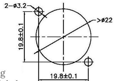
Available in 3 or 5 pin, Male or Female variations with options for vertical or horizontal PCB mounting.
