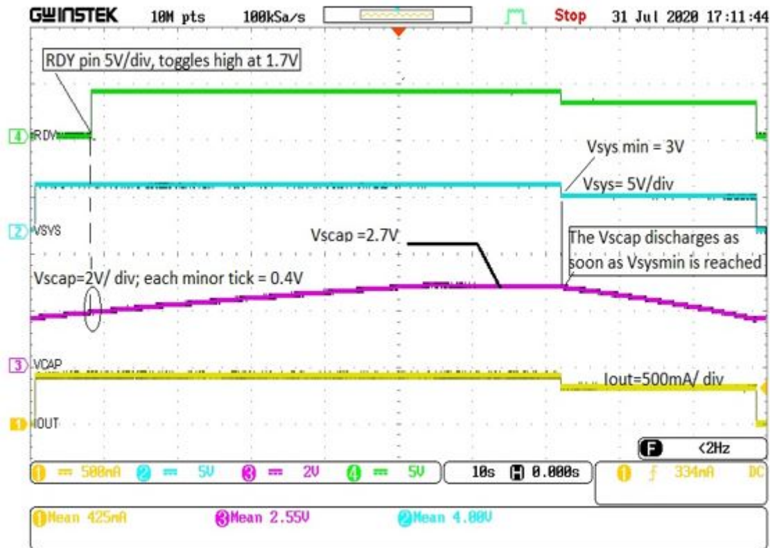
Figure 5: The MAX38888 is ready for discharge from V_{SCAP} = 1.7V . Since FET (M1) is on, charges all way to 2.7V.
