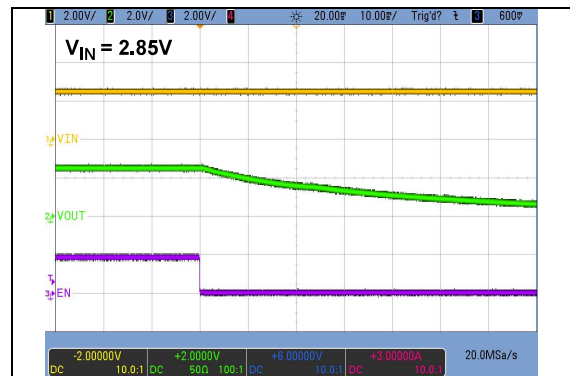
FIGURE 2-11: Turn-Off with Enable.
