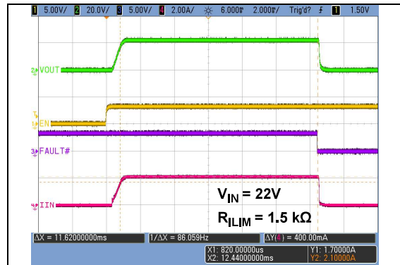
FIGURE 2-4: Overcurrent Fault Response Delay Time.
