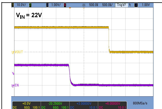
FIGURE 2-2: V_{OUT} Fall Time.
