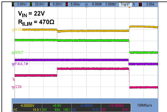
FIGURE 2-25: Current Overload Response.
