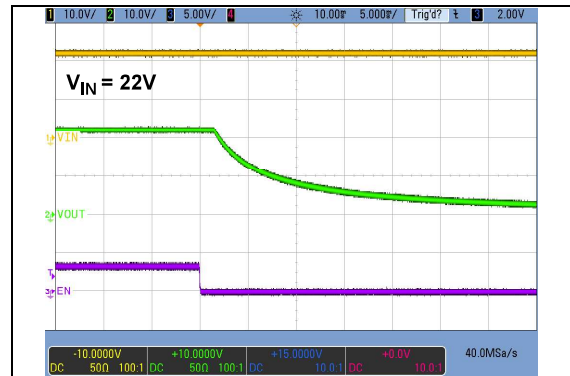
FIGURE 2-12: Turn-Off with Enable.
