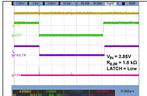
FIGURE 2-16: Output Recovery from Short Circuit.
