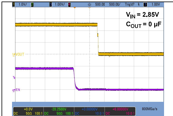
FIGURE 2-1: V_{OUT} Fall Time.
