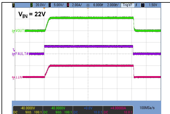
FIGURE 2-14: Turn-On Into 20% Overload.
