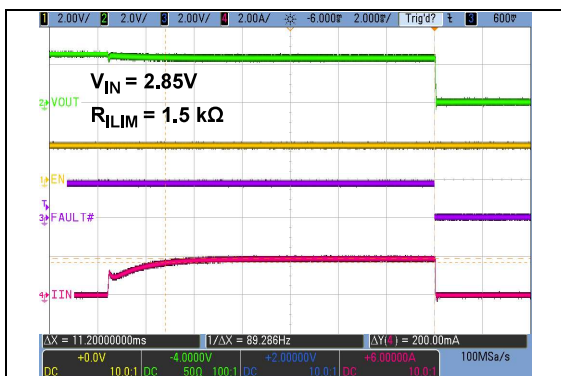
FIGURE 2-3: Overcurrent Fault Response Delay Time.
