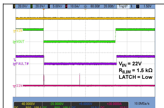
FIGURE 2-17: Output Recovery from Short Circuit.
