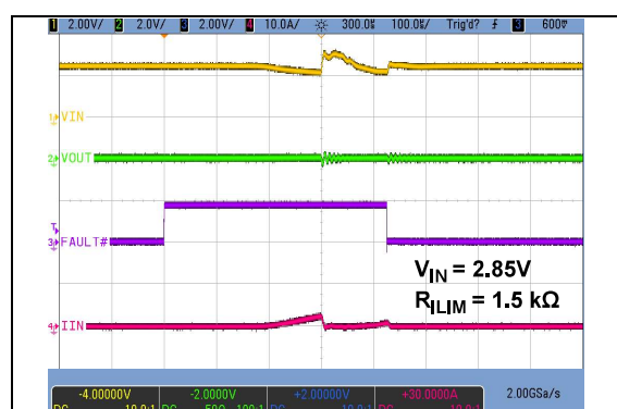
FIGURE 2-18: Turn-On into Short to GND.
