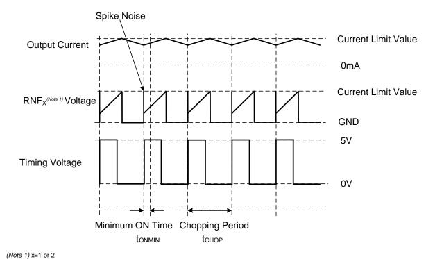
Figure 1. Timing chart of TIMING voltage, RNF<sub>x</sub> voltage and output current
