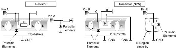
Figure 9. Example of monolithic IC structure
