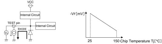
Figure 3. Model diagram for measuring chip temperature
