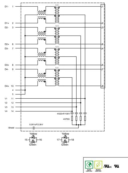
CHECKED REVISION DATE (YYYY-MM-DD) GENERAL TOLERANCE PROJECTION METHOD JefL 001.000 2020-05-12 DIN ISO 2768-1m DESCRIPTION WE-RJ45 LAN Transformer 1000 Würth Elektronik eiSos GmbH & Co. KG Base-T, PoE+ ORDER CODE EMC & Inductive Solutions Max-Eyth-Str. 1 7499510440 74638 Waldenburg Germany Tel. +49 (0) 79 42 945 - 0 www.we-online.com STATUS BUSINESS UNIT PAGE WÜRTH ELEKTRONIK 2/6 eiSos Valid eiSos@we-online.com
