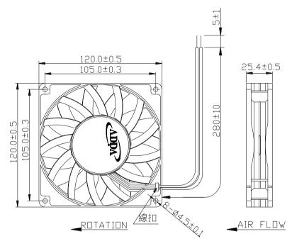
LEAD WIRES: UL 1007, AWG24, L = 280±10 mm Red = positive; Black = negative.
