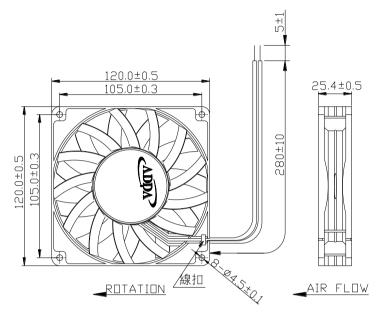
LEAD WIRES: UL 1007, AWG24, L = 280±10 mm Red = positive; Black = negative.
