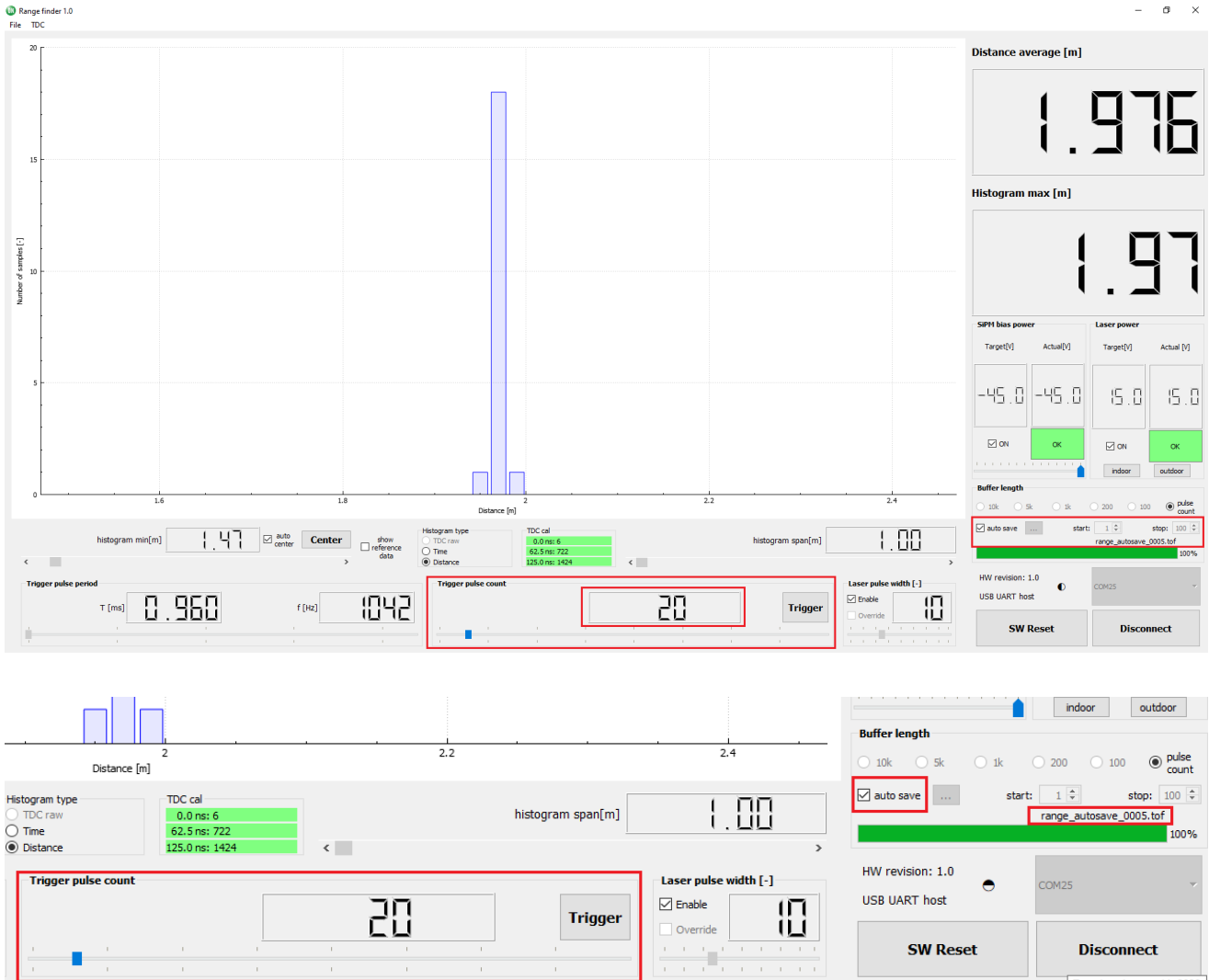
Figure 19. Auto Saving of Measured Data in Trigger Mode
