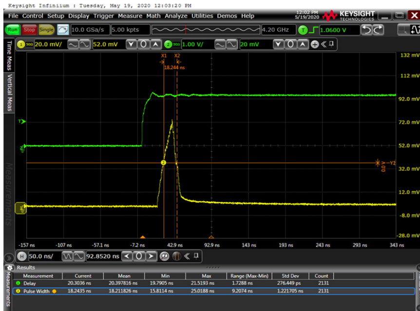
Figure 40. Typical Laser Optical Pulse Shape
