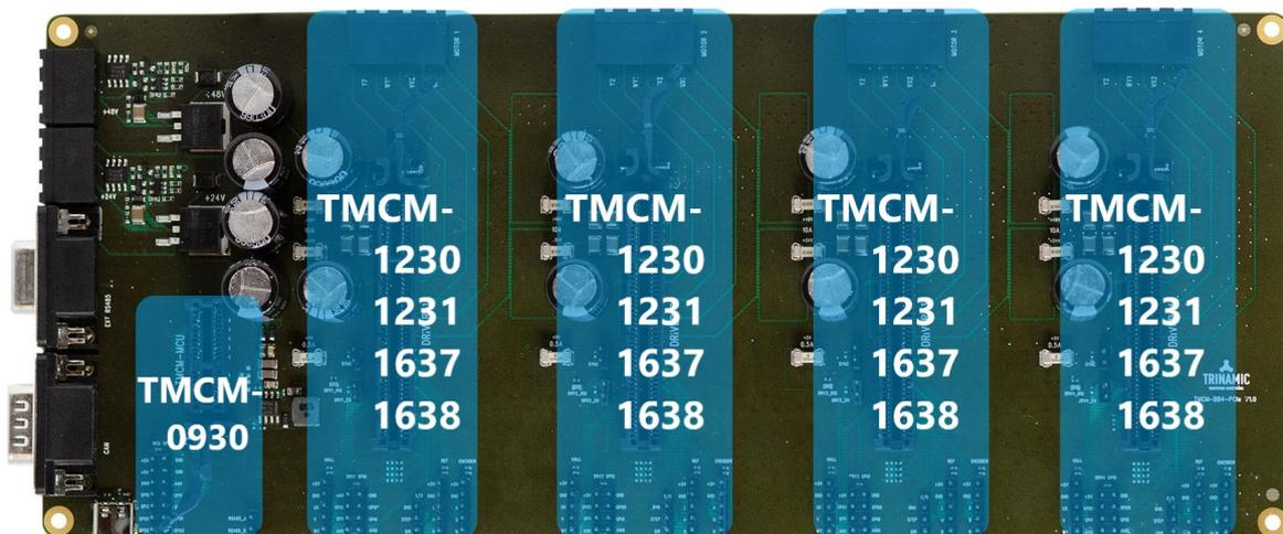
Figure 1: TMCM-BB4 Base board with available slots
