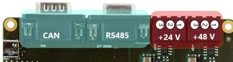
Figure 3: Power; Communication and USB-C connectors of TMCM-BB4
