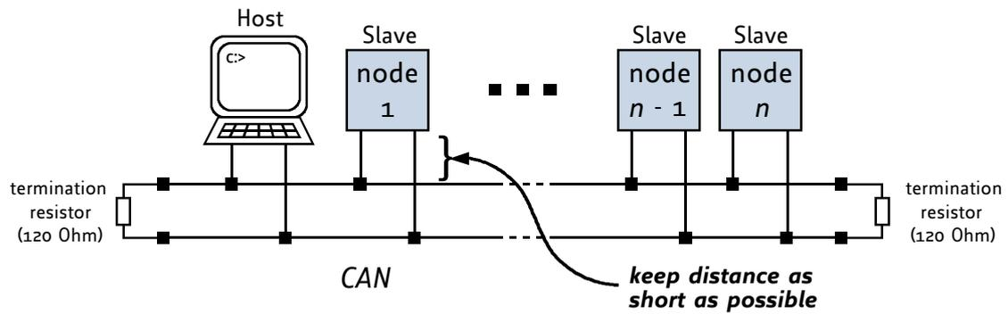
Figure 8: CAN bus structure with termination resistors
