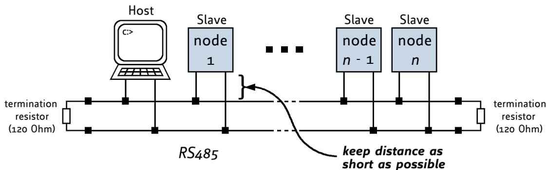
Figure 5: RS485 bus structure with termination resistors
