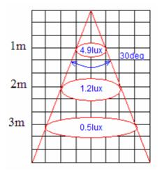
These values have been calculated using the efficiency values of the lens listed above and the formula  $\mathbf{E} = \mathbf{I} / \mathbf{d}^2$ , where  $\mathbf{E}$  is the irradiance in lux,  $\mathbf{I}$  the intensity in cd, and  $\mathbf{d}$  the distance between the lens output and the measured point.
