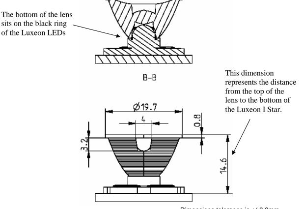
Dimensions tolerance is +/-0.2mm
