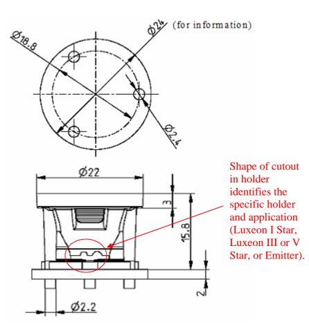
Dimensions tolerance is +/-0.2mm
