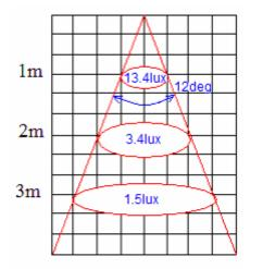
With FLP-HMB3-LL-y: Low Profile Medium Beam lens for Lambertian Luxeon LEDs
