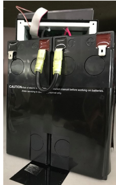
Step 6: Disconnect the jumper between the battery packs.
