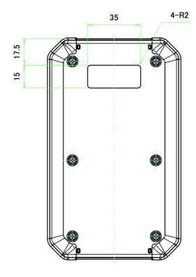
Maximum Carrier Board Dimensions (mm):
