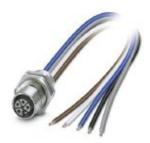
Flush-type connector, Power, 5-position, Socket, M12, L - Power, Rear mounting, M16 x 1.5, Individual wires, cable length: 0.2 m, 1.31 mm², UL/cUL stranded hook-up wire
