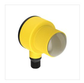
T30R R-GAGE Series Radar Sensor Range 15 m; Input 10-30 V dc 0-10 V Analog, 1 NPN/PNP Configurable with IO Link 5 Pin Euro (M12) 150 mm Pigtail Quick Disconnect Part Number: 808902
