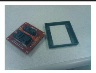
1. Remove the top cover from the socket module.
