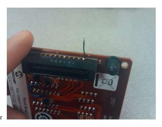
3. Now, run the wire thru the top of the P2 connector as shown in the picture.
