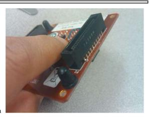
4. Bend the tip of the wire and hook it to the outmost top pin in the P2 connector as shown in the picture.
