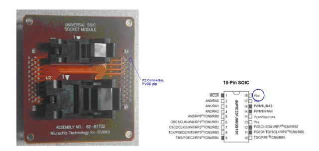
The goal is to provide the PVDD high-current voltage source directly to the VDD (pin 18) of the 18P SOIC device. Keep in mind that the 18-pin SOIC will be top-justified inside the 28P socket of the PM3 socket module.
