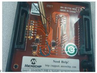
2. Solder the wire at the bottom of the socket module to the 28-SOIC socket pin 28, DUT pin 18 (VDD).
