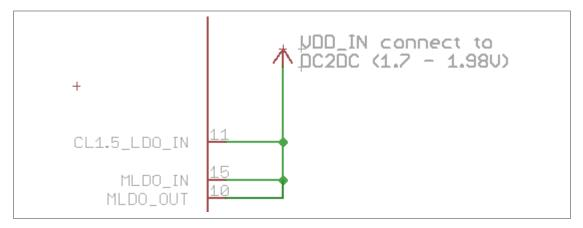
Mixed DC2DC- $V_{BAT}$  system (Maximum RF output power and optimum system power, but requires routing of  $V_{BAT}$ ):
