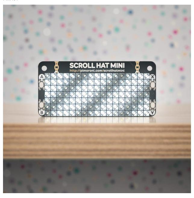
A 17x7 matrix of bright white LEDs with individual brightness control, and four handy buttons, made for
