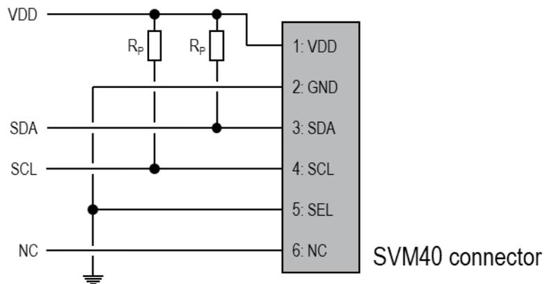
**Figure 2** Typical I<sup>2</sup>C application circuit to connect the SVM40 sensor module.
