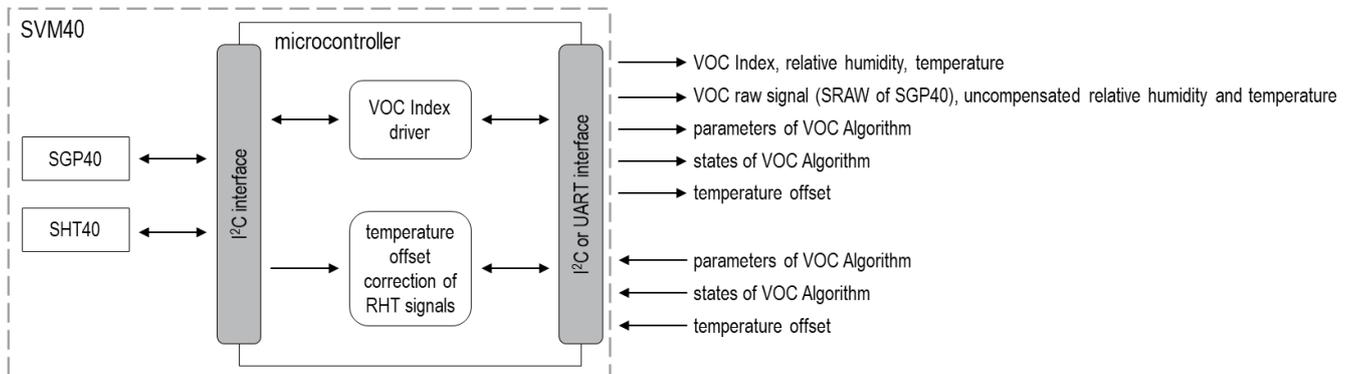
**Figure 1** Schematic of the signal processing and interface on SVM40.
