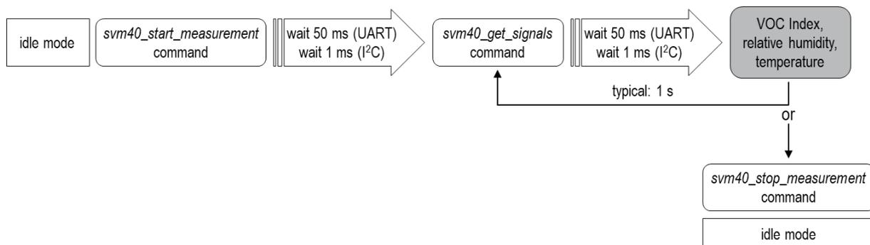
**Figure 5** Process flow for performing a measurement including raw signals with the SVM40 to receive VOC Index, relative humidity, temperature, SGP40 raw signal (SRAW), uncompensated relative humidity, and uncompensated temperature.
