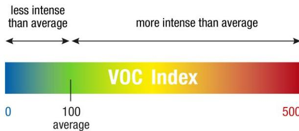
**Figure 6** Explanation of the VOC Index scale.
