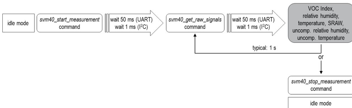
**Figure 4** Process flow for performing a standard measurement with the SVM40 to receive VOC Index, relative humidity, and temperature.
