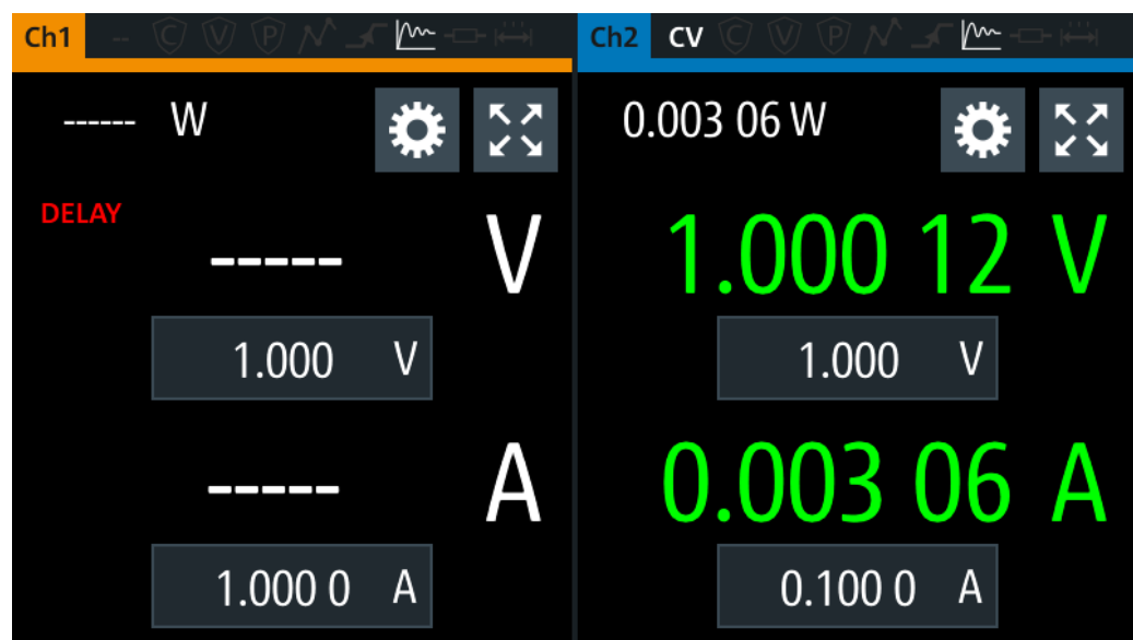
Figure 6-8: Delay text at channel display area
