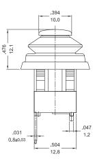
Dimensions: Inches/Millimetres Tolerances ±0.012"/0.3mm
