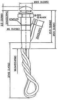
Dimensions : Millimetres (Inches) Tolerances ±0.3mm (0.012")
