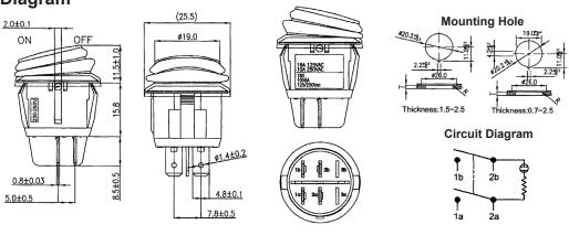
Dimensions : Millimetres Tolerances ±0.3mm
