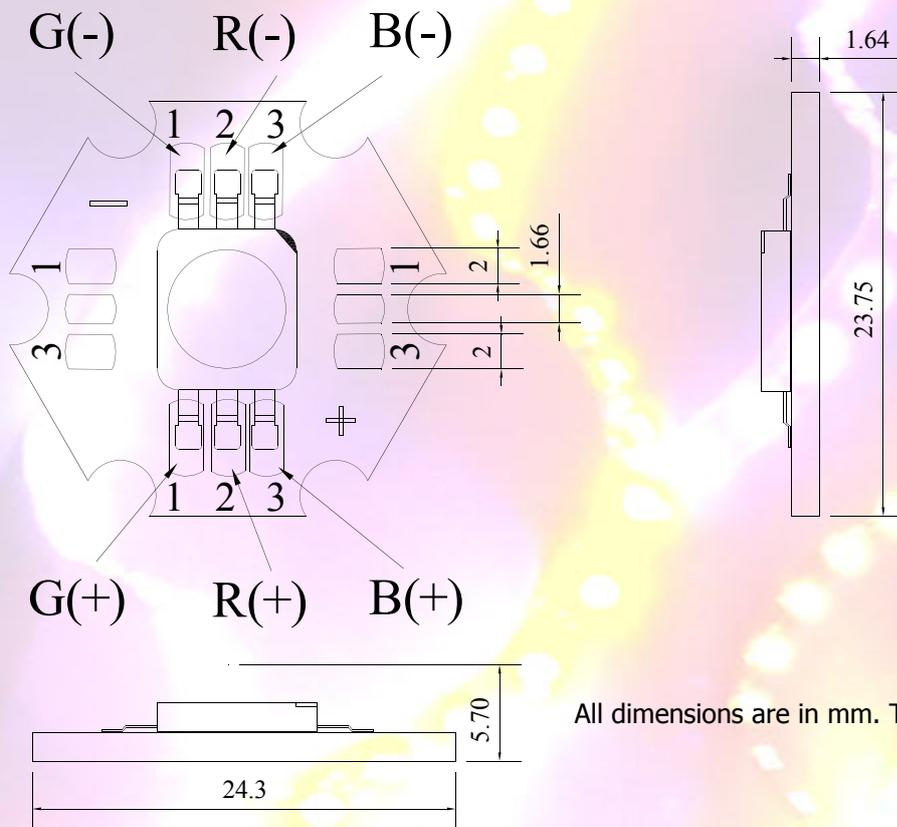
All dimensions are in mm. Tolerance  $\pm 0.5$ mm.
