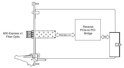
Figure 1-8. NI PXI-8368 (157298x-02L) Block Diagram
