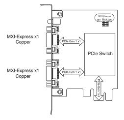
Figure 1-5. NI PXI-8360 (191373x-01) Block Diagram
