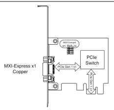
Figure 1-4. NI PCIe-8362 (190735x-01L) Block Diagram
