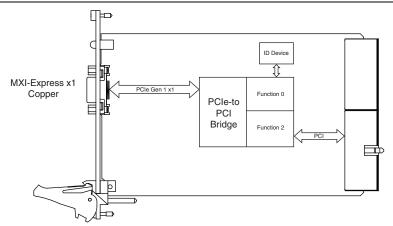
Figure 1-6. NI PXI-8364 (199991x-02L) Block Diagram
