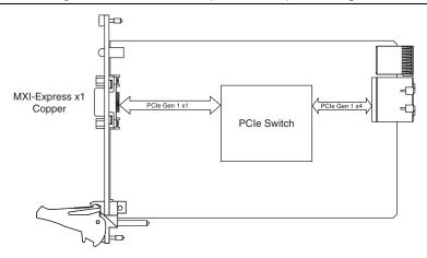
Figure 1-11. NI ExpressCard-8360 (198266x-01L) Block Diagram
