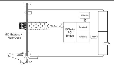
Figure 1-9. NI PXIe-8360 (194402x-01L) Block Diagram
