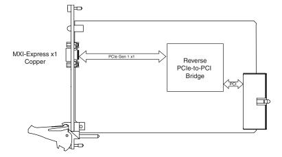
Figure 1-7. NI PXI-8367 (199991x-04L) Block Diagram
