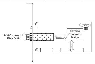
Figure 1-3. NI PCIe-8361 (199042x-01L) Block Diagram
