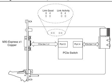
**Link Good LEDs**—LEDs that indicate a successful cable link (LED 0) and backplane link (LED 4).
