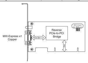
Figure 1-2. NI PCI-8366 (199392x-02L) Block Diagram
