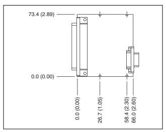
Figure 1. NI 9208E Dimensions in Millimeters (Inches)
