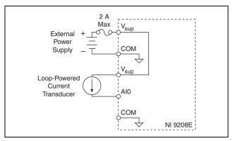
Figure 4. Connecting a Loop-Powered Current Transducer to the NI 9208E
