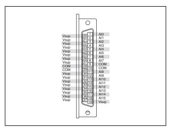
Figure 2. NI 9208E Pin Assignments
