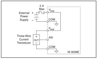
Figure 5. Connecting a Three-Wire Current Transducer to the NI 9208E
