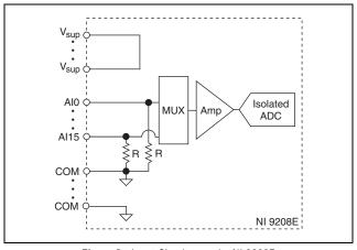
Figure 3. Input Circuitry on the NI 9208E
