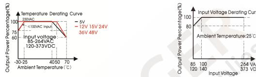
Note: 1.With an AC input voltage between 85 -100VAC and a DC input between 120-140VDC the output power must be derated as per the temperature derating curves:
