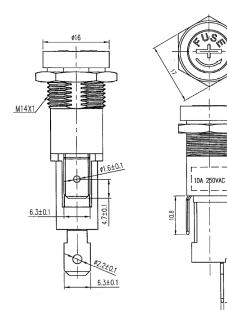
Dimensions : Millimetres Tolerance ±0.3mm
