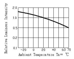
Luminous Intensity vs. Ambient Temperature
