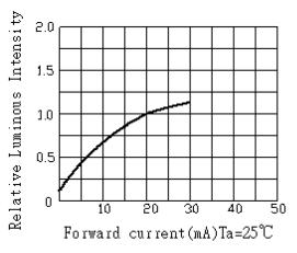
Luminous Intensity vs. Forward current
