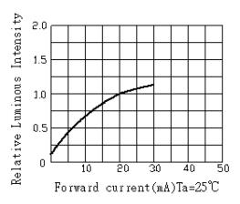
Luminous Intensity vs. Forward current
