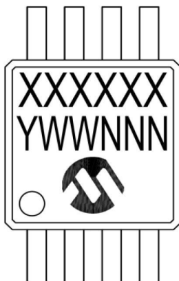
10-Lead MSOP (3 x 3 mm)
