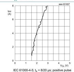
Fig. 7. Dynamic resistance with positive clamping; typical values
