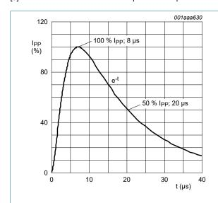
8/20 µs pulse waveform according to Fig. 1. IEC 61000-4-5
