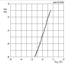
IEC 61000-4-5;  $t_p$  = 8/20  $\mu$ s; positive pulse **Dynamic resistance with negative clamping**;
