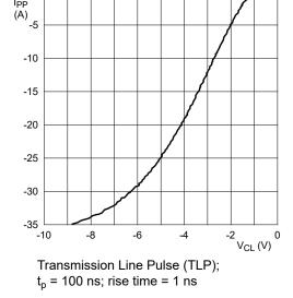
Fig. 6. Dynamic resistance with negative clamping; typical values
