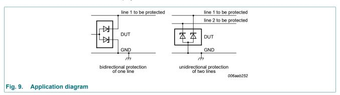
The device uses an advanced clamping structure showing a negative dynamic resistance. This snap-back behavior strongly reduces the clamping voltage to the system behind the ESD protection during an ESD event. Do not connect unlimited DC current sources to the data lines to avoid keeping the ESD protection device in snap-back state after exceeding breakdown voltage (due to an ESD pulse for instance).
