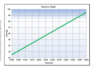
Stroke & force values are measured using spring pins with an internal construction per the design specification. Individual spring pin performance may vary from these values based on design differences.
