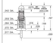
Standard Tolerances: Lengths: ±.006 Diameters: ±.002
