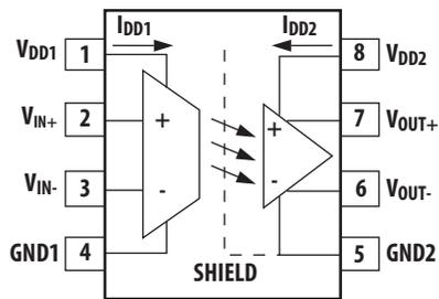
**NOTE:** A 0.1  $\mu\text{F}$  bypass capacitor must be connected between pins 1 and 4 and between pins 5 and 8.
