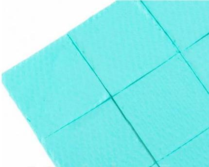
Laird Tflex™ HD80000 is the latest product in the High Deflection gap filler series. Tflex™ HD80000 combines 6 W/mK thermal conductivity with superior pressure versus deflection characteristics. The combination will allow minimal stress on components while also yielding low thermal resistance. As a result, less mechanical and thermal stresses will be experienced within your device.
