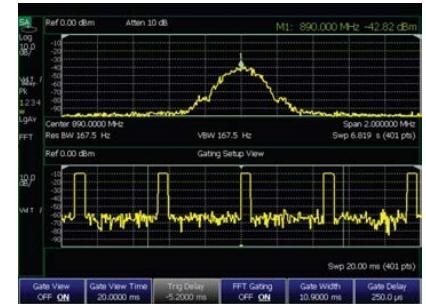
Analyze pulsed RF signals using the time-gating option
