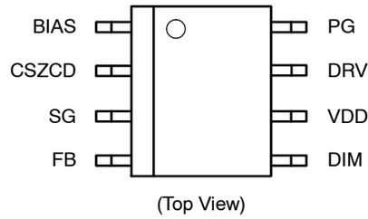
Figure 3. Pin Configuration
