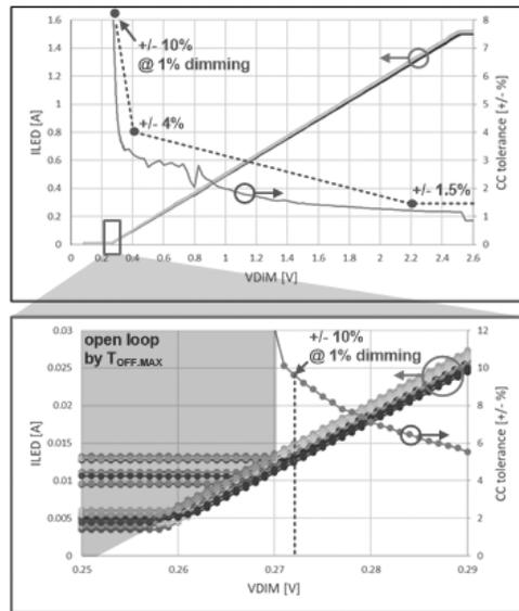
Figure 12. NCL35076 Dimming Curve and CC Tolerance
