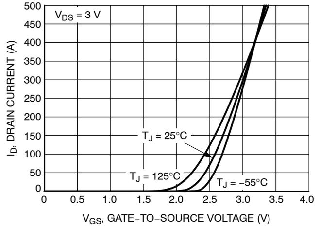
Figure 2. Transfer Characteristics
