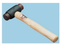
$\label{lem:main_main} \textbf{Malleable iron head fitted with both faces of rawhide which are replaceable when worn. Widely used throughout industry.}$
