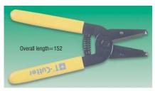
A wire cutter with shear type blades which leaves a clean cut edge with the absolute minimum of crushing-no more oval ends! It easily cuts solid copper and aluminium conductors up to  $6 \mathrm{mm}^2$  and finely stranded cable of much greater diameter. Slim design.
