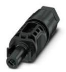
Photovoltaic connector, Range of articles: PV-CF-C, Photovoltaic connector, housing material: PPE, color: black, number of positions: 1, min. conductor cross section: 2.5 mm², max. conductor cross section: 6 mm², nom. voltage: 1500 V, rated current: 27 A, Connection method: Crimp, Type of contact: Socket, min. cable diameter: 5.00 mm, max. cable diameter: 8.00 mm
