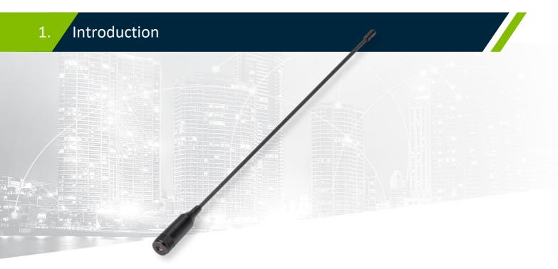
The FW.24 is a flexible 2.4GHz whip antenna with a SMA(M) connector for outdoor use. It features excellent efficiency (>75%) and high peak gain (>4 dBi) between 2400-2500MHz on a 30\*30cm ground plane.
