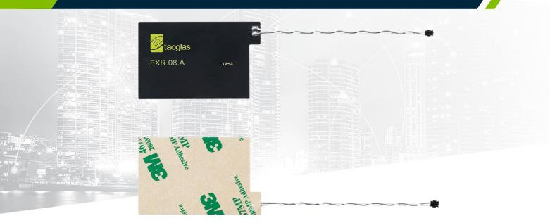
The FXR.08.52.0075X.A is a rectangular, flexible, NFC (Near Field Communications) antenna for use in mobile devices and other applications such as keycards, payment systems, and boarding passes. The design provides a flexible NFC antenna with 75mm twisted pair 28AWG cable that can be adhered to the plastic enclosure of the device for ease of installation and work with specific 13.56MHz RFID and NFC chips which need to connect via JST ACH connector.
