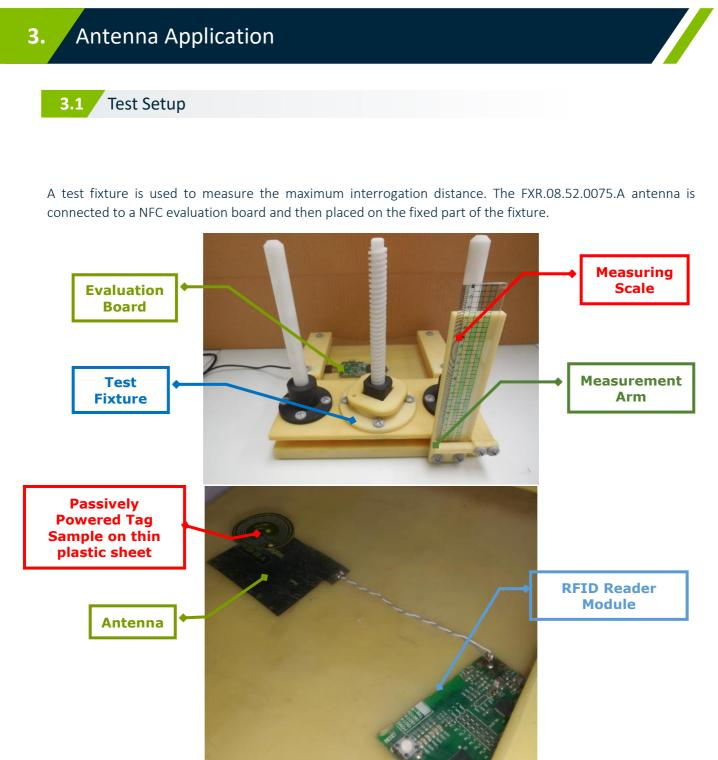
The test sample is placed on a thin sheet of plastic connected to the movable part of the fixture. Then the distance is carefully adjusted until the reader can no longer read the sample, thus the maximum interrogation distance is displayed in the ruler.
