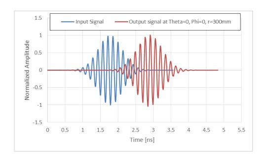
Fidelity of signals as above is calculated and results as below are obtained. The values are well above 0.9 and it is considered that antenna has very good performance.
